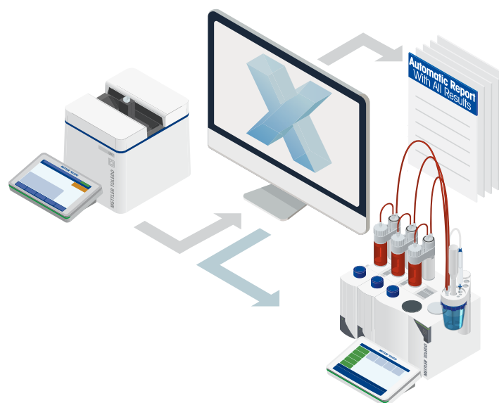
Figure 1: Schematic of multiparameter setup with titration and UV/Vis spectroscopy.
